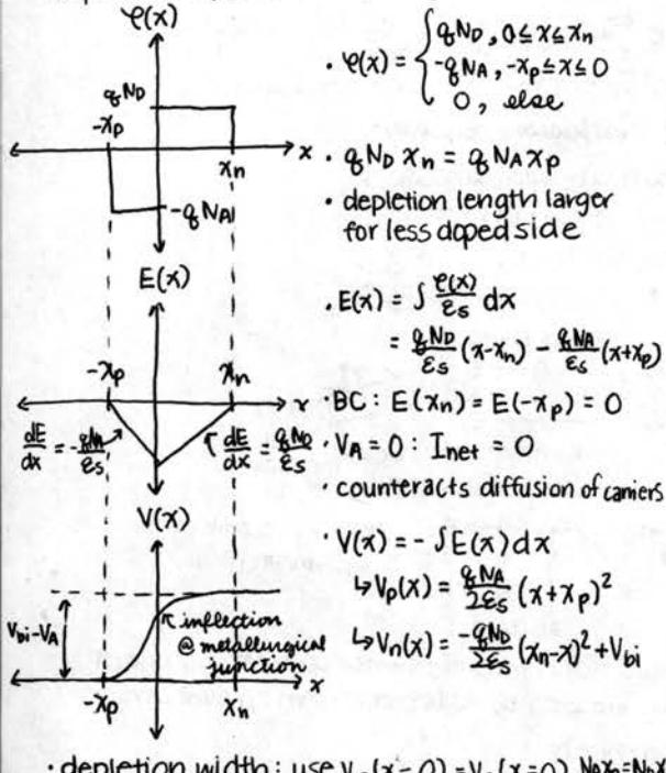
$$\begin{aligned} &\text{depletion width: use } V_n(x=0) = V_p(x=0), N_A x_p = N_D x_n \\ &\hookrightarrow x_p = \left[ \frac{2e(V_{bi}-V_A)}{q} \left( \frac{N_D}{N_A} \frac{1}{N_D + N_A} \right) \right]^{1/2} \\ &\hookrightarrow x_n = \left[ \frac{2e(V_{bi}-V_A)}{q} \left( \frac{N_A}{N_D} \frac{1}{N_D + N_A} \right) \right]^{1/2} \\ &\hookrightarrow W = x_p + x_n = \left[ \frac{2e(V_{bi}-V_A)}{q} \left( \frac{1}{N_A} + \frac{1}{N_D} \right) \right]^{1/2} \end{aligned}$$
