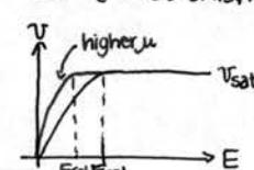
$$\cdot I_{DS} = \begin{cases} \text{long-channel } I_{DSat} & , lin + LC \\ 1 + \frac{V_{DS}}{E_{sat} L} & , sat LC \\ \text{long-channel } I_{DSat} & , sat SC \\ 1 + \frac{V_{DS} - V_T}{m E_{sat} L} & , sat SC \\ W \tau_{sat} \mu_{eff} (V_{GS} - V_T) & , sat SC \\ \frac{W}{2} E_{sat} & \Downarrow I_{DSat} \propto (V_{GS} - V_T, not L) \\ I_{DSat} \neq L & \end{cases}$$
