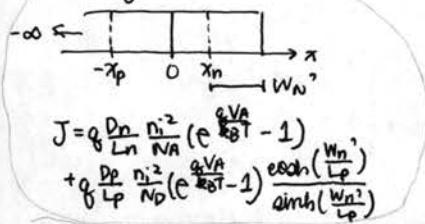
$$J = q \frac{D_n}{L_n} \frac{n_i^2}{N_A} (e^{\frac{qV_A}{kT}} - 1) \frac{\cosh(\frac{w_n}{L_n})}{\sinh(\frac{w_n}{L_n})} + q \frac{D_p}{L_p} \frac{n_i^2}{N_D} (e^{\frac{qV_A}{kT}} - 1) \frac{\cosh(\frac{w_p}{L_p})}{\sinh(\frac{w_p}{L_p})}$$
