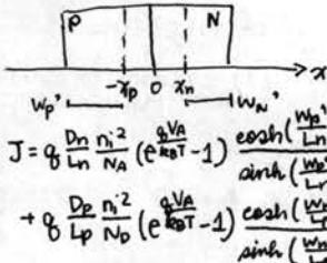
$$J = q \frac{D_n}{L_n} \frac{n_i^2}{N_A} (e^{\frac{qV_A}{kT}} - 1) \frac{\cosh(\frac{w_p}{L_n})}{\sinh(\frac{w_p}{L_n})} + q \frac{D_p}{L_p} \frac{n_i^2}{N_D} (e^{\frac{qV_A}{kT}} - 1) \frac{\cosh(\frac{w_n}{L_p})}{\sinh(\frac{w_n}{L_p})}$$
