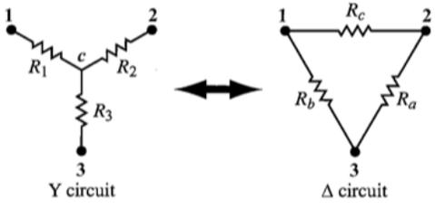
$$R_1 = \frac{R_b R_c}{R_a + R_b + R_c} \quad R_a = \frac{R_1 R_2 + R_2 R_3 + R_1 R_3}{R_1}$$
